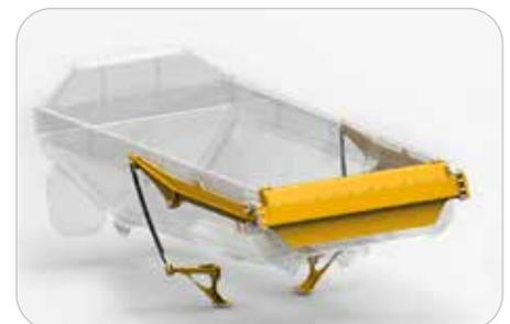
A tailgate is available as an option for better material retention. The tailgate opens as the bin is raised for dumping. Spring steel straps maintain positive seal throughout the haul, ensuring minimal material is lost.
