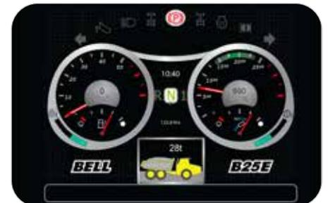
The exclusive on-board weighing presents the operator with real time information on the payload while the machine is being loaded. A 'speed restriction' mode can also be activated if the machine is significantly overloaded.
