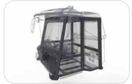
Our quiet operator cabins are ROPS/ FOPS certified with an air suspension operator seat. The trainer seat has a retractable lap belt while the operator seat has a standard 3 point seat belt. Both have automatically locking retractors.
