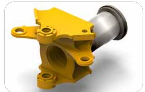
High-strength steel and widely spaced taper roller bearings in the articulation area enhance long-term durability.
