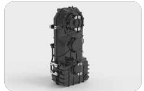
The transfer case inter-axle differential delivers equal torque to each axle when traction is favorable. When conditions deteriorate, the diff-lock automatically engages to deliver torque to the tires that can best use it.
