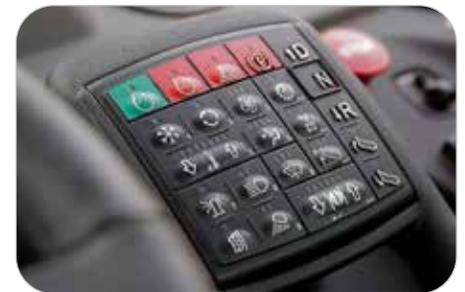
Keyless start, driver identity and access codes ensure no unauthorized operation of your equipment.
